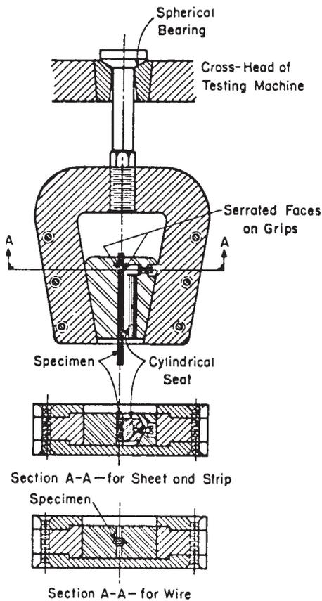
FIG. 4 Gripping Devices for Sheet and Wire Specimens
