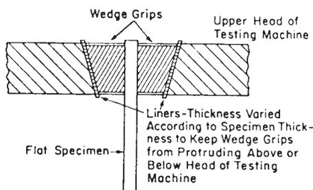
FIG. 1 Wedge Grips with Liners for Flat Specimens
