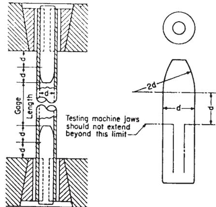
NOTE 1—The diameter of the plug shall have a slight taper from the line limiting the testing machine jaws to the curved section.
