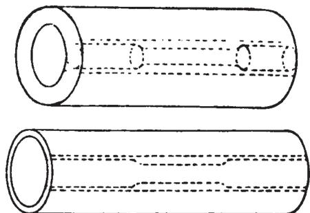
NOTE 1—The edges of the specimen shall be cut parallel to each other.
